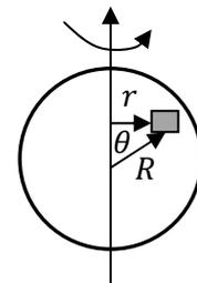
$$I = \int_{casca} r^2 dm = \int_{casca} [R \sin(\theta)]^2 \rho R^2 \sin(\theta) d\theta d\phi = \rho R^4 \int_0^\pi [\sin(\theta)]^3 d\theta \int_0^{2\pi} d\phi$$
